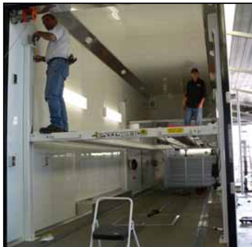
16 FOOT CAR LIFT BEING INSTALLED INTO H&H BIGBRUTE
