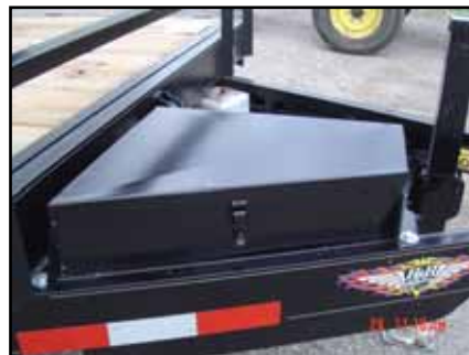
Tongue mounted toolbox for MX and EX SpeedLoader models.
