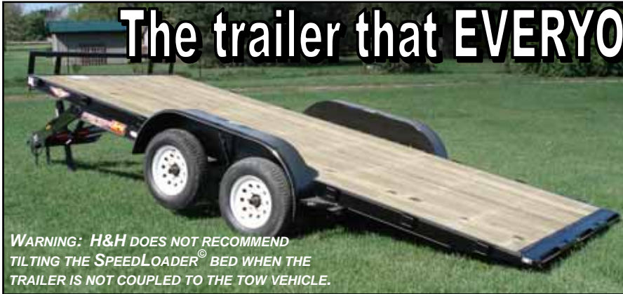
WARNING: H&H DOES NOT RECOMMEND TILTING THE SPEEDLOADER ® BED WHEN THE TRAILER IS NOT COUPLED TO THE TOW VEHICLE.
